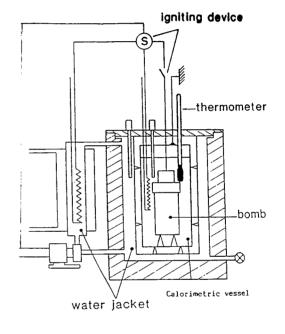
Fig.2 Scheme of the apparatus used for testing according to EN ISO 1716
