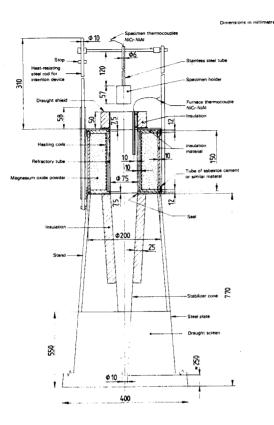
Fig. 1. Apparatus for testing non-combustibility according to EN ISO 1182
