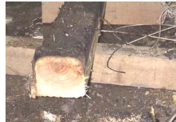
Figure 7: Carbonization depth of the post around part of each specimen (mm).
