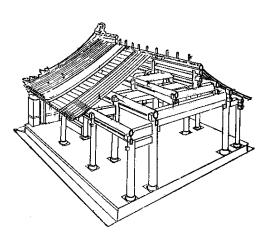
Figure 1: The wood structural frame of historical buildings in China.
