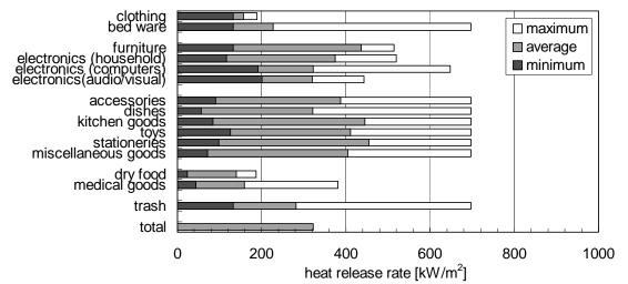
Figure 16 Heat Release Rate Values for Each Group of Combustibles
