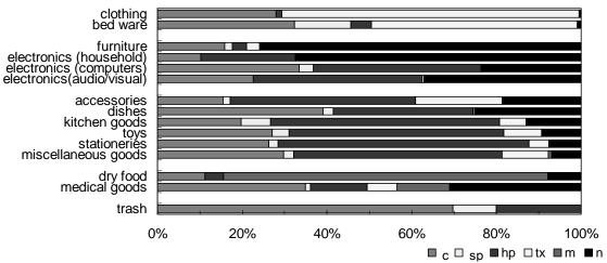
Figure 14 Weight Fraction of Constituents (c=cellulose, sp = soft plastics, hp = hard plastics, tx = textile materials, m = miscellaneous materials, n = non-combustible materials)
