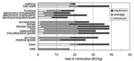
Figure 15 Heat of Combustion Values for Each Group of Combustibles
