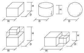
Figure 1 Definition of characteristic dimension of combustible items
