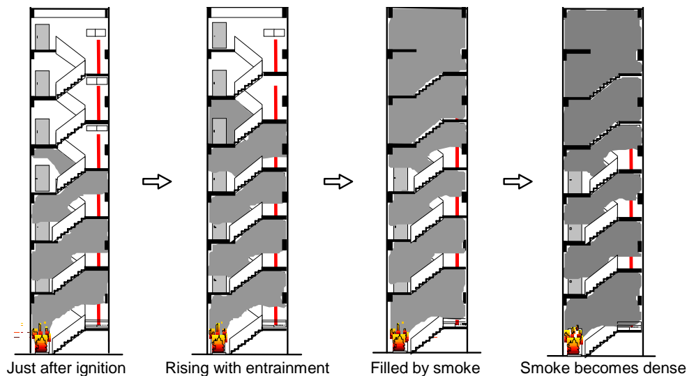
FIGURE 4. Schematics of smoke rising in case of no opening above fire source
