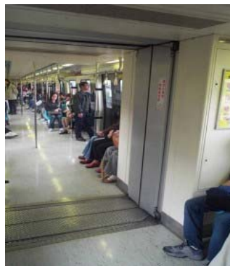
Figure 3. The construction of coupling between cars in Taipei MRT
