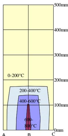
Figure 12: Max temperature distribution (Case1).
