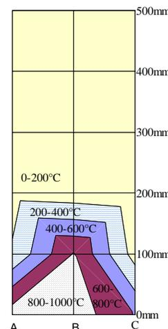
Figure 15: Max temperature distribution (Case4).
