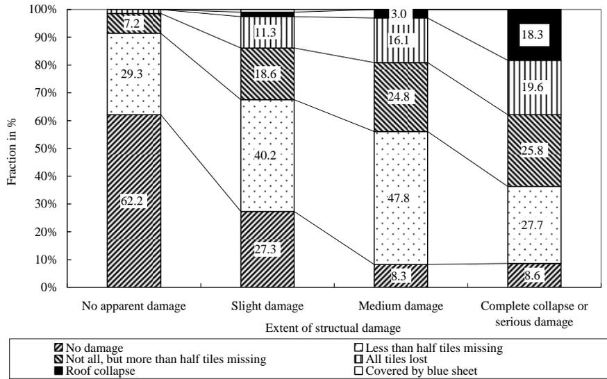
Figure 4.2: Roof tile deficit according to the extent of structural damage (fraction in %) (for all areas (Areas 1-6)).
