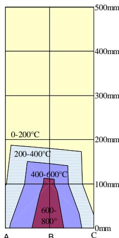
Figure 13: Max temperature distribution (Case2).
