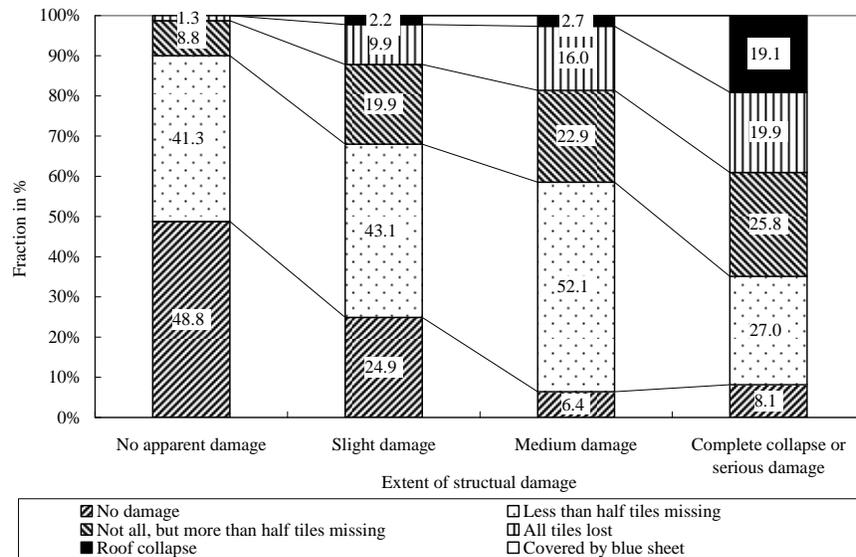
Figure 3.2: Roof tile deficit according to the extent of structural damage (fraction in %) (for severely damaged areas (Areas 2, 5, 6)).
