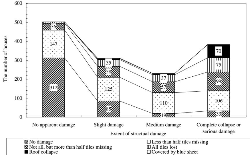
Figure 4.1: Roof tile deficit according to the extent of structural damage (the number of houses) (for all areas (Areas 1-6)).
