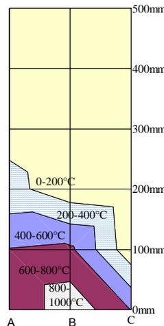
Figure 14: Max temperature distribution (Case3).
