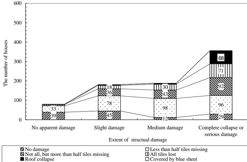
Figure 3.1: Roof tile deficit according to the extent of structural damage (the number of houses) (for severely damaged areas (Areas 2, 5, 6)).
