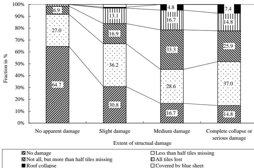
Figure 2.2: Roof tile deficit according to the extent of structural damage (fraction in %) (for less damaged areas (Areas 1, 3, 4)).
