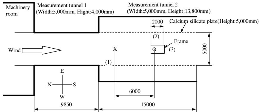
Figure 5: Layout in Fire Wind Tunnel (unit: mm).
