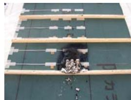
Photo 6: Damage on the surface (Case 1).
