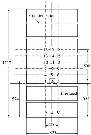
Figure 6: Top face of test roof (unit: mm).
