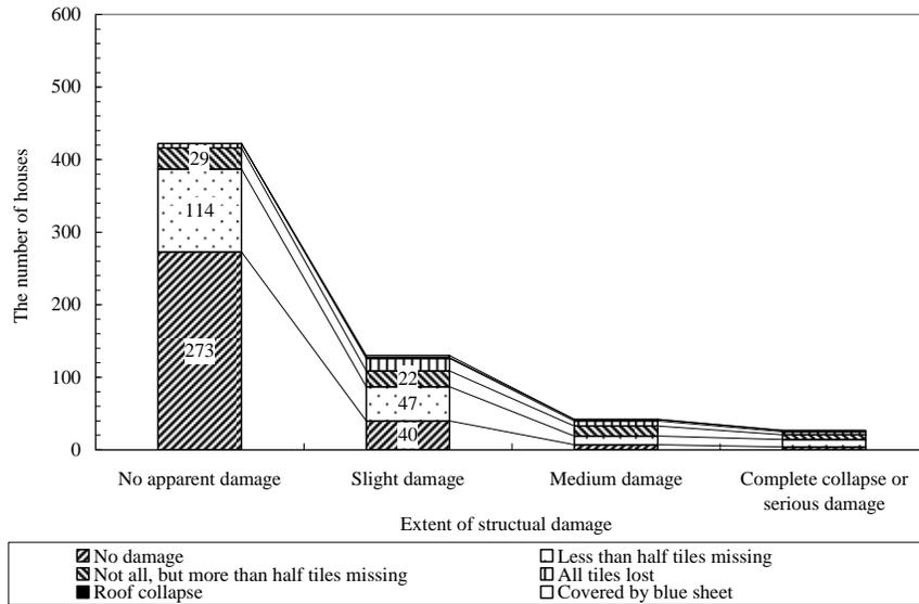
Figure 2.1: Roof tile deficit according to the extent of structural damage (the number of houses) (for less damaged areas (Areas 1, 3, 4)).
