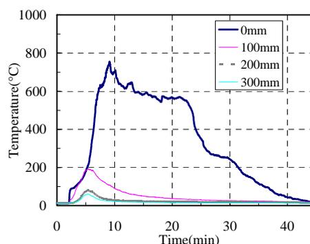
Figure 9: Surface temperature along line B (Case 2).
