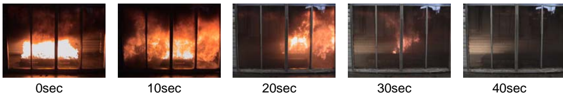
Figure 15. Photographs of behavior of fire during fire suppression in Test E-3
