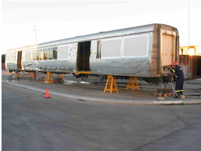
Figure 1. Carriage shell used for fire experiments
