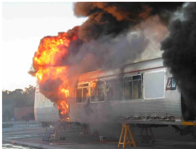
Figure 5. Fire plume through doorway from fully developed fire
