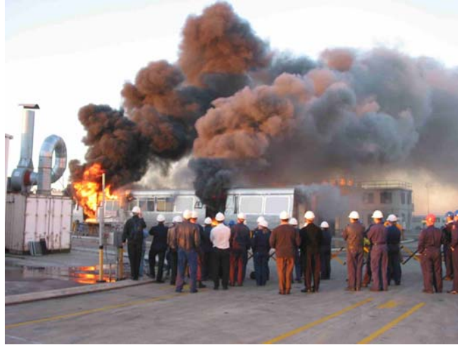
Figure 4. Smoke production from fully developed fire
