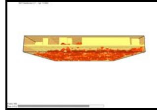
■ Smoke layer descent in Plenum area (415s)
