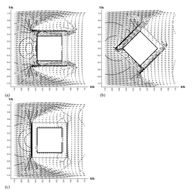
**FIGURE 2.** Normalised velocity vector distribution and contour lines of pressure coefficient over the symmetry horizontal flow plane of the refuge floor which is located at the building mid-height with a large square-planned main services core located at its centre: (a) Wind blowing at normal incident to the building (stream-wise), (b) Wind blowing at an angle diagonally to the building, and (c) Wind blowing at an angle perpendicular to the solid side walls of the refuge floor
