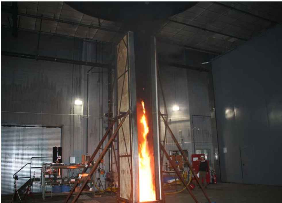
FIGURE 12. Non-fire-propagating panels in the parallel panel test
