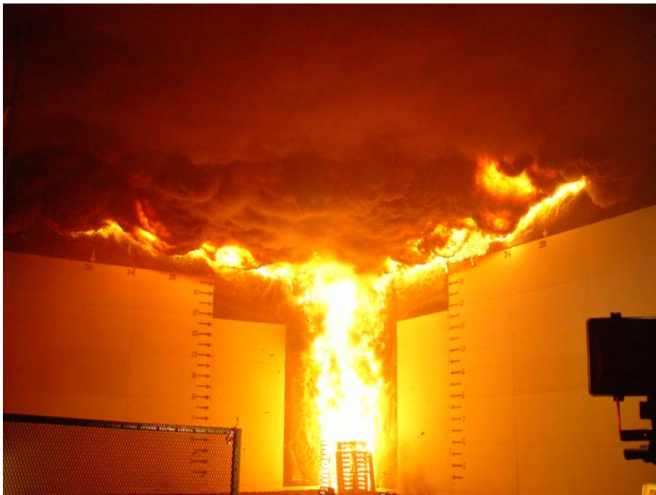
FIGURE 3. Fire propagating panels in the 25 ft corner test
