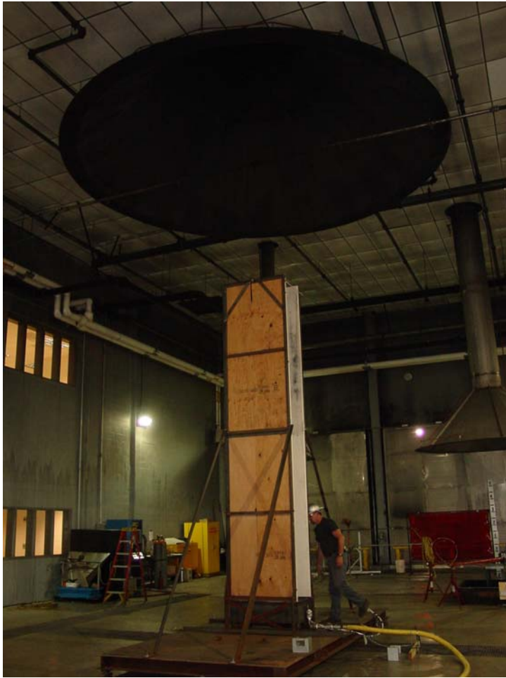
FIGURE 9. Photo showing the 4.9 m high parallel panel test apparatus under the 5 MW fire products collector
