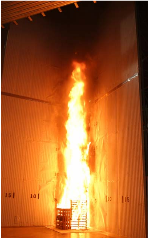
FIGURE 6. Non-fire-propagating panels in the 50 ft corner test
