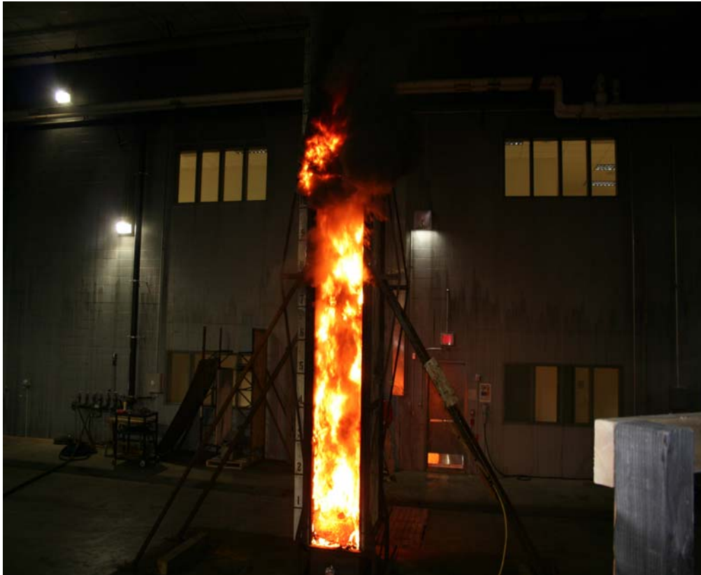
FIGURE 11. Fire-propagating panels in the parallel panel test
