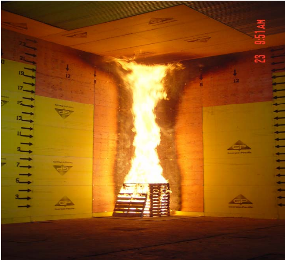
FIGURE 4. Non-fire-propagating panels in the 25 ft corner test
