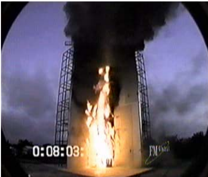
FIGURE 5. Fire propagating panels in the 50 ft corner test
