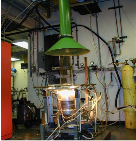
FIGURE 1a. Fire propagation apparatus (FPA) FIGURE 1b. Combustion of sample at FPA
