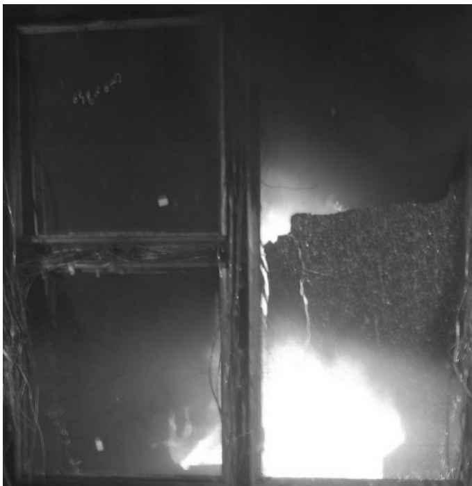
FIGURE 14. Breakage and fallout of toughened glass
