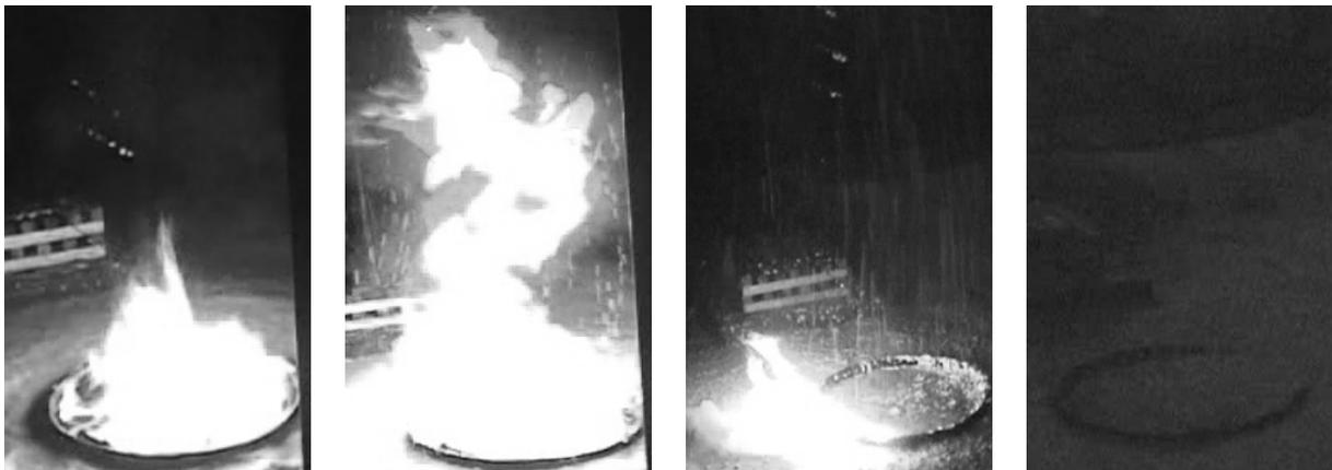
(1) 15s after ignition (2) 60s after ignition, injection started (3) 13s after injection (4) 17s after ignition
