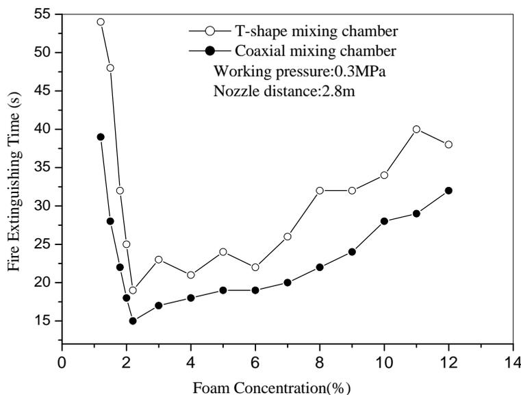
**FIGURE 3.** Effects of mixing chamber structure on fire extinguishments
