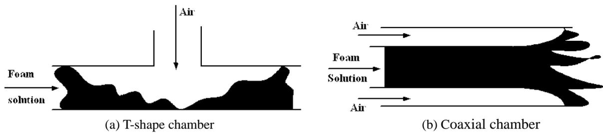
**FIGURE 2.** Schematic diagram of the mixing chamber
