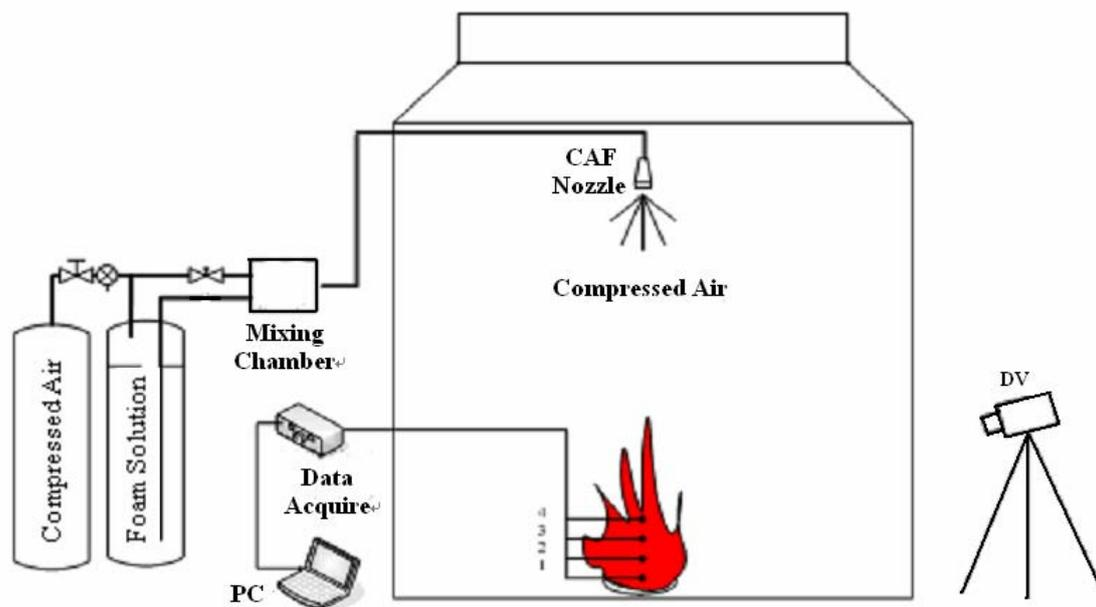
**FIGURE 1.** Schematic diagram of the experimental apparatus
