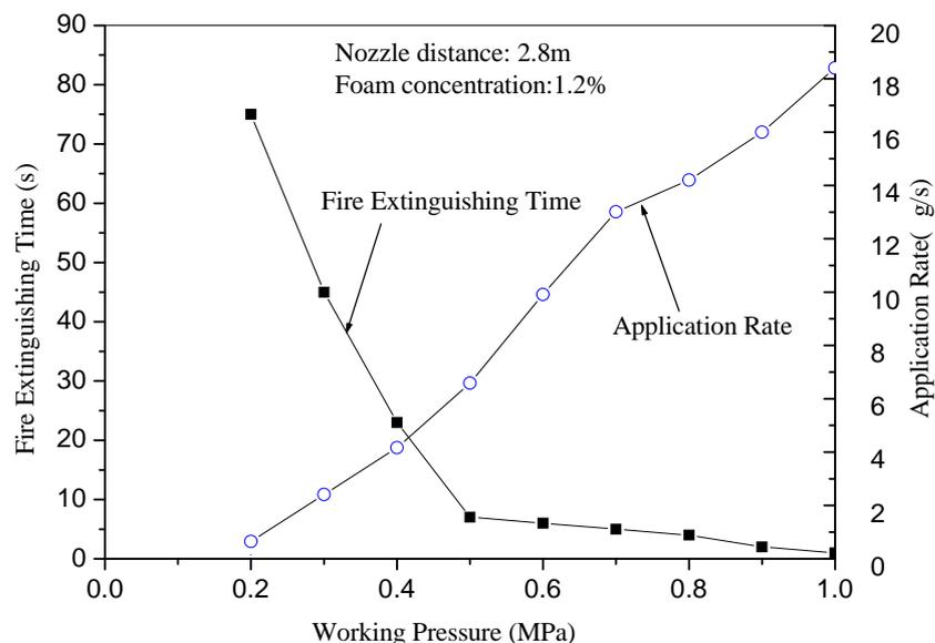
**FIGURE 7.** Effects of working pressure on fire extinguishments
