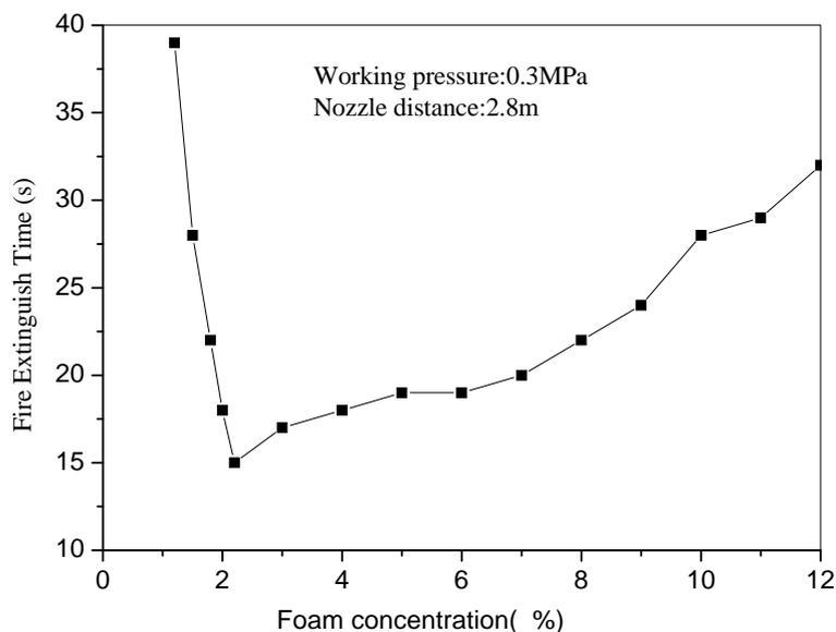
**FIGURE 4.** Effects of foam concentration on fire extinguishments
