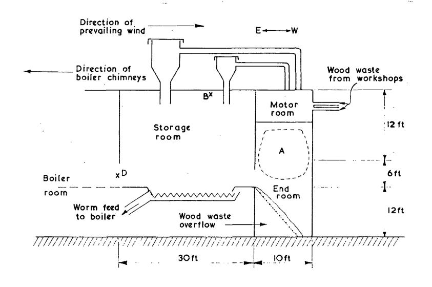
FIG. 1. SECTIONAL SKETCH OF BUILDING IN WHICH EXPLOSION OCCURRED
