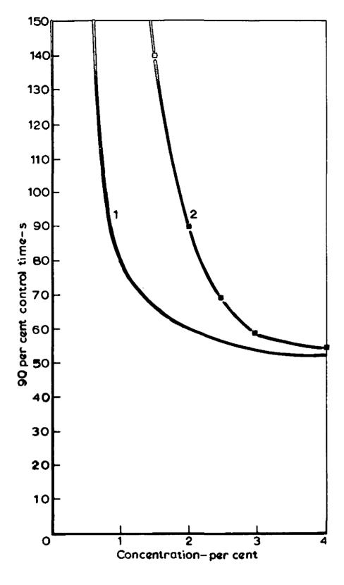
1=0.28m² area fires of 62-68°C boiling range petrol-application rate=  $2.4 \, \text{C/m}^2$ -min-gentle surface application-from Fire Research Note 933 2=0.25m² area fires of aviation gasoline application rate= $3 \, \text{C/m}^2$ -min forceful application
