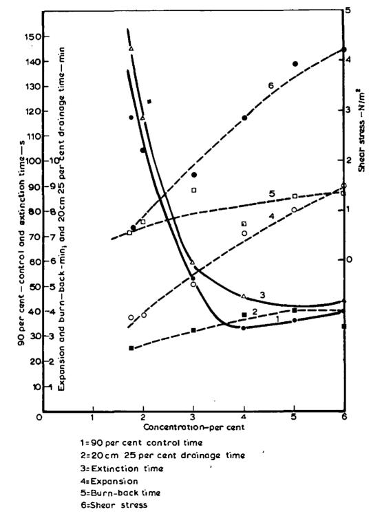
Figure 1 0.25 m<sup>2</sup> area petrol fires extinguished with fluorochemical foam applied at 3 l/m<sup>2</sup>-min and used with various concentrations
