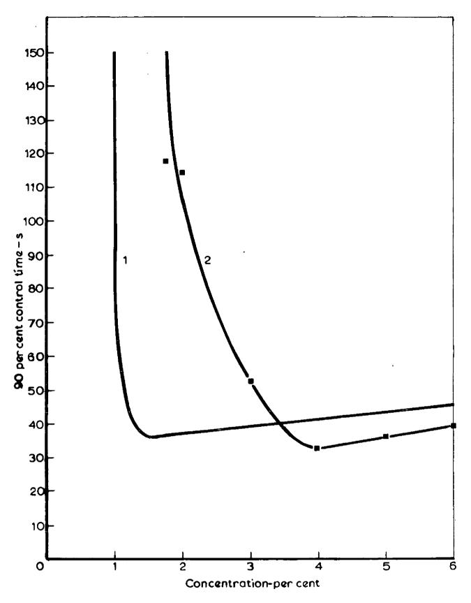
1=0.28m² area tires of 62-68°C boiling point petrol - application rate = 2.4 Um²-min - gentle surface application - from Fire Research Note 933 2=0.25m² area fires of aviation gasoline - application rate 3 Um²-min forceful application
