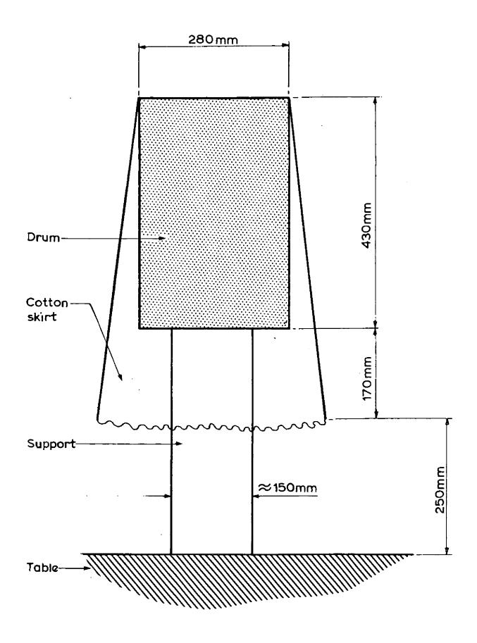
Figure 1'Clothing fire' fabric and drum dimensions
