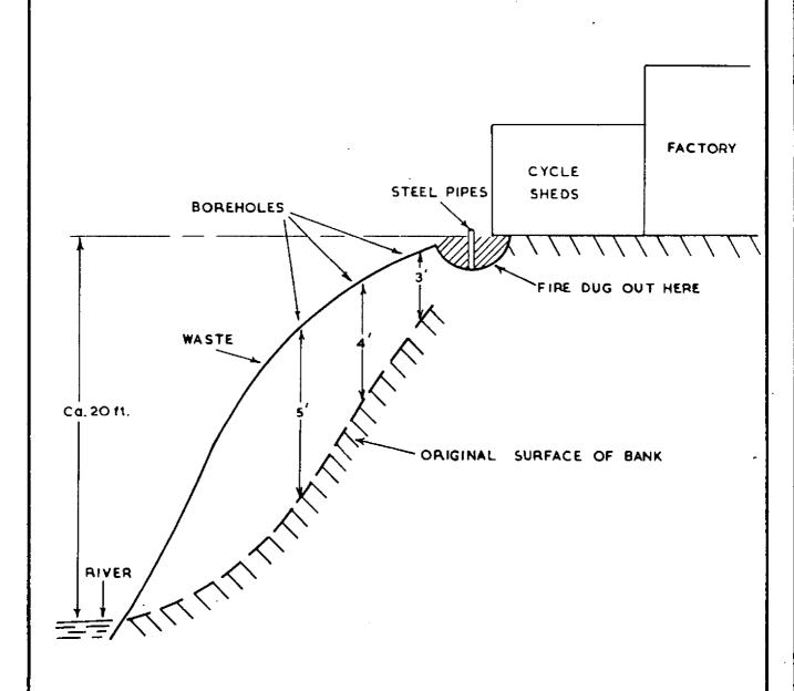
FIG. 1. PROBABLE CROSS SECTION OF SITE.
