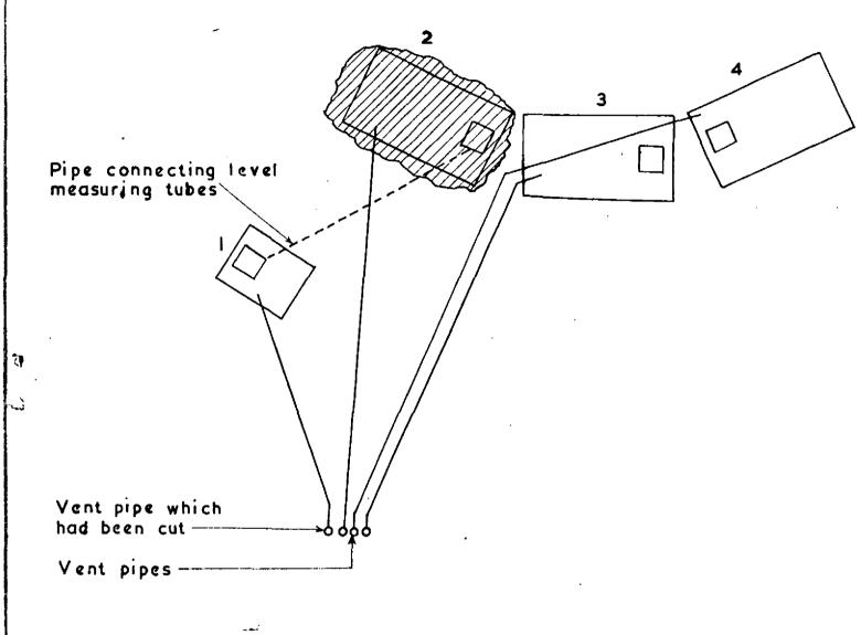
FIG. 2. RELATIVE POSITION OF TANKS ON THE SITE.
