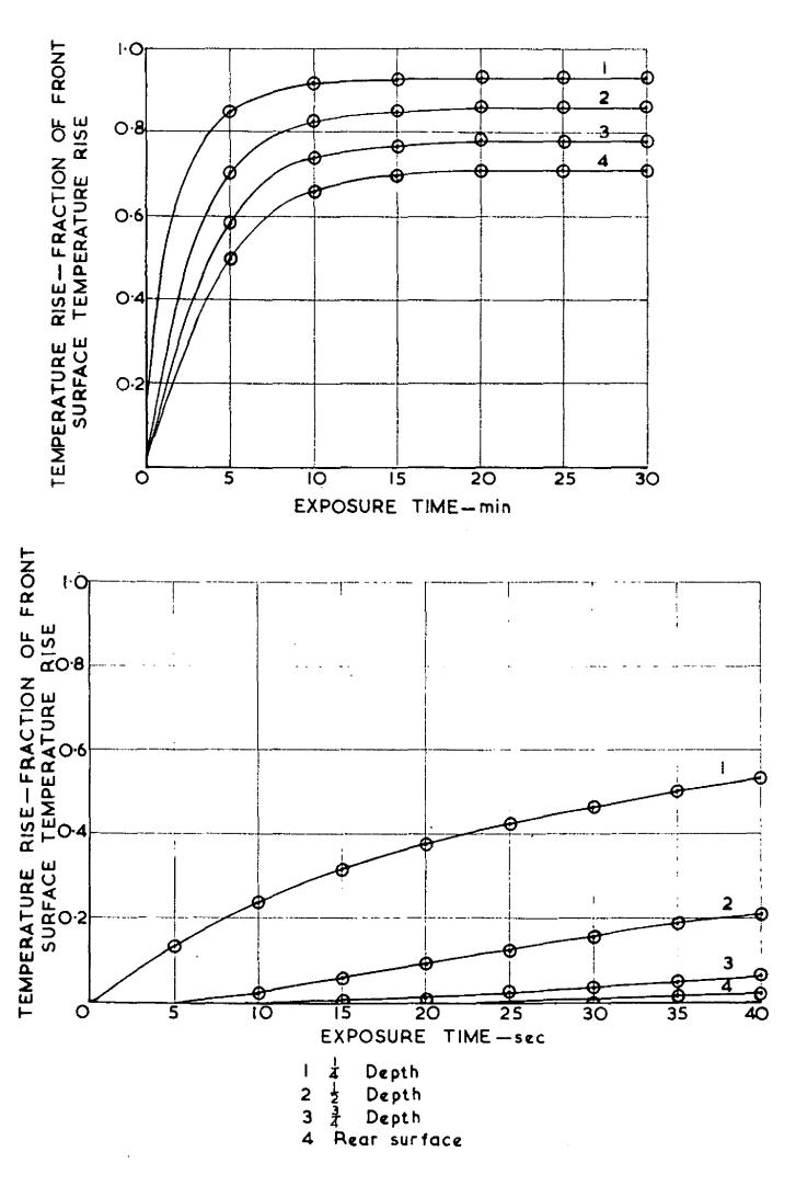
FIG. 1. CASE I. TEMPERATURE RISE AT DIFFERENT DEPTHS EXPRESSED AS A FRACTION OF THE APPLIED FRONT SURFACE TEMPERATURE RISE.
