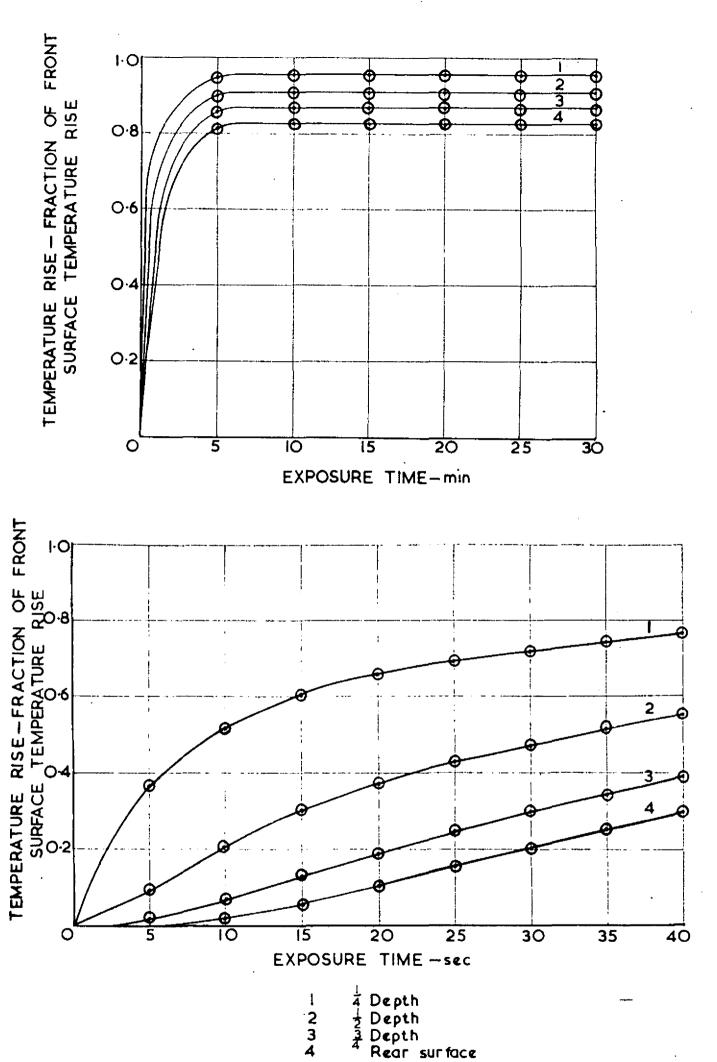
FIG. 3. CASE III. TEMPERATURE RISE AT DIFFERENT DEPTHS EXPRESSED AS A FRACTION OF THE APPLIED FRONT SURFACE TEMPERATURE RISE.
