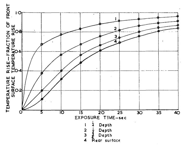
FIG. 2. CASE II. TEMPERATURE RISE AT DIFFERENT DEPTHS EXPRESSED AS A FRACTION OF THE APPLIED FRONT SURFACE TEMPERATURE RISE.
