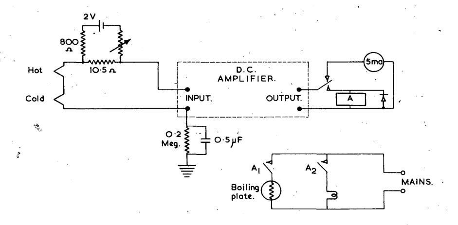
FIG. 1. CIRCUIT OF TEMPERATURE CONTROL UNIT FOR BOILING PLATE.
