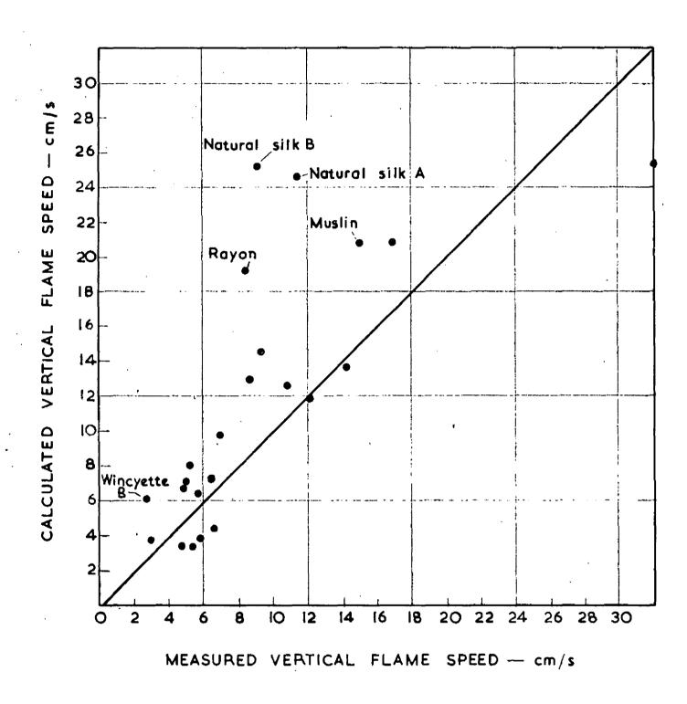
FIG.3. CALCULATED & OBSERVED VERTICAL FLAME SPEED FROM AMERICAN TEST
