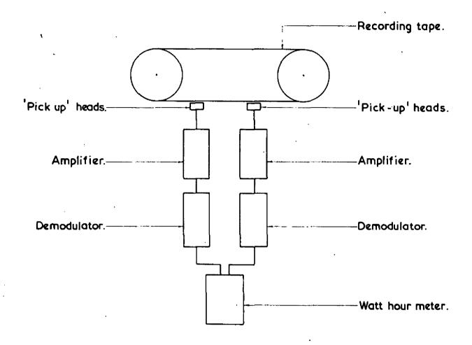
FIG. 2. A SCHEMATIC OF A AUTOCORRELOGRAM
