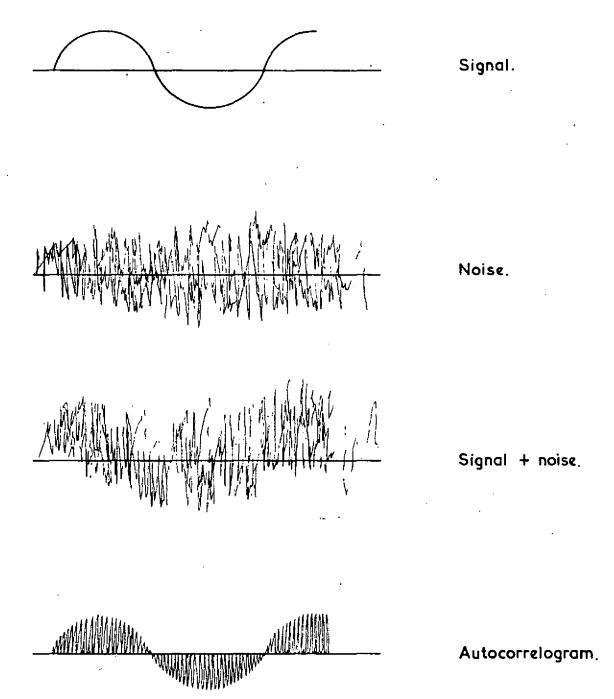
FIG.I. A SIGNAL AND ITS AUTOCORRELOGRAM.
