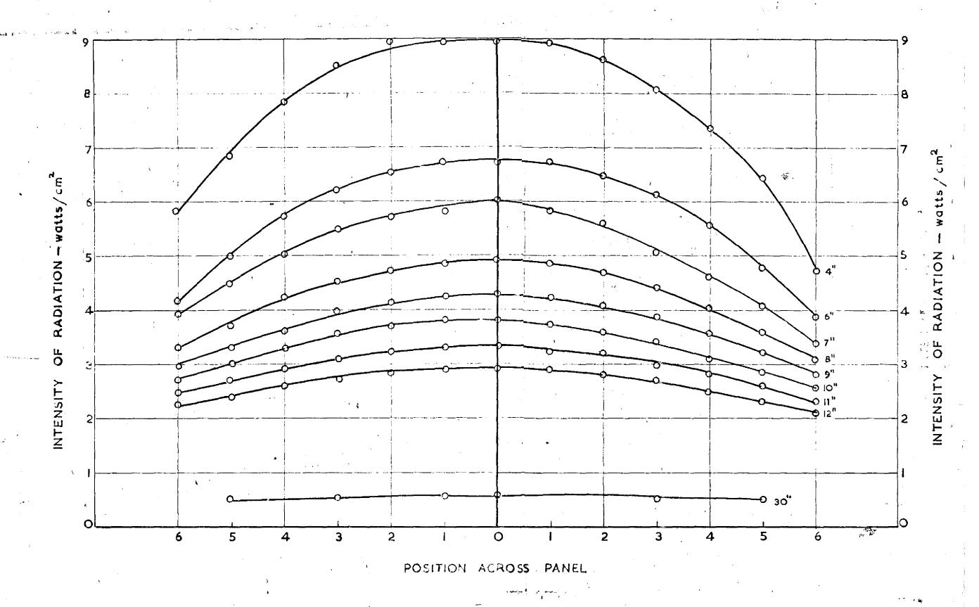
FIG.2. DISTRIBUTION OF RADIATION IN HORIZONTAL PLANE THROUGH CENTRE OF PANEL
