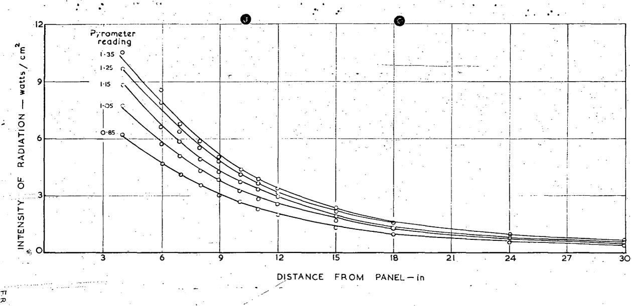
FIG. 4 DISTRIBUTION OF RADIATION ALONG CENTRAL AXIS OF PANEL FOR DIFFERENT PANEL TEMPERATURES
