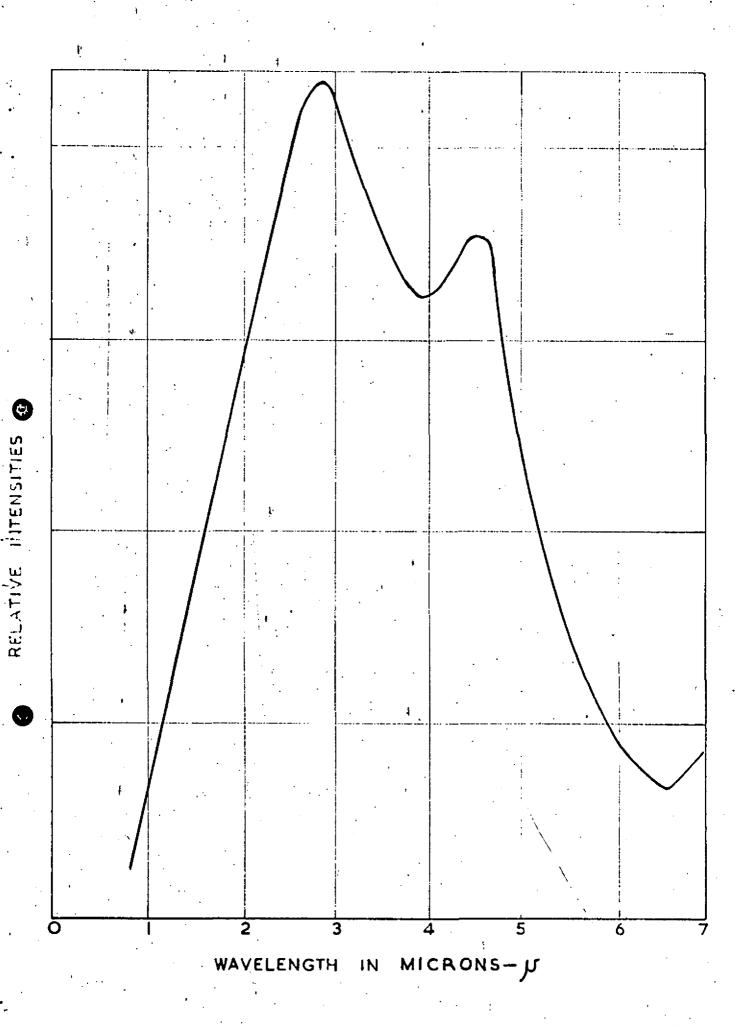
FIG.I. SPECTRAL EMISSION OF A RADIANT PANEL 870°C
