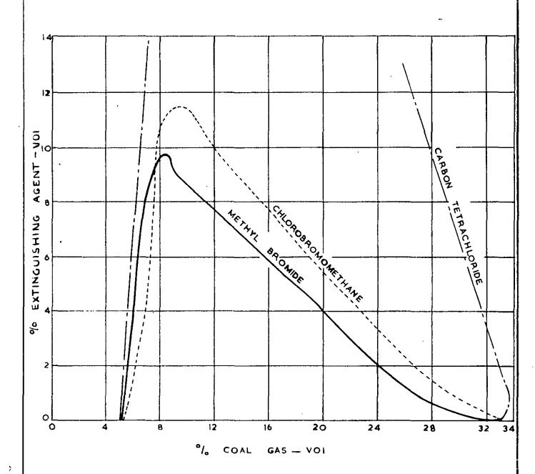
FIG.I. INFLAMMABILITY LIMITS OF COAL GAS WITH AIR AND ADDITIONS OF EXTINGUISHING AGENTS.
