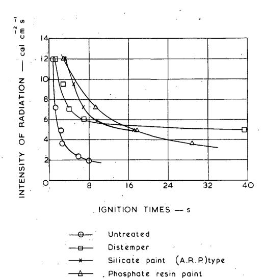
FIG.I. IGNITION TIMES FOR TREATED
