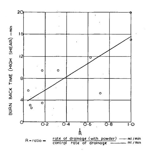
FIG.4 RELATIONSHIP BETWEEN THE BURN BACK TIME AND THE RECIPRICAL OF THE N.R.L. TEST RATIO
