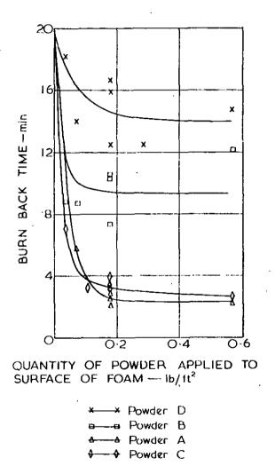
FIG. 2. THE EFFECT ON THE STABILITY OF FOAM OF THE APPLICATION OF POWDER TO ITS SURFACE
