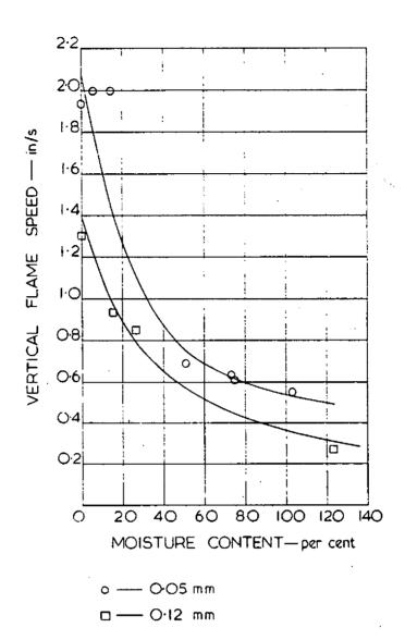
FIG. 2. VARIATION OF VERTICAL FLAME SPEED WITH MOISTURE CONTENT
