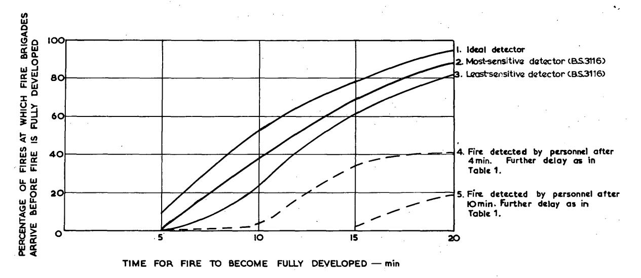
FIG. I. EFFICIENCY OF AUTOMATIC FIRE DETECTORS - RURAL COUNTIES
