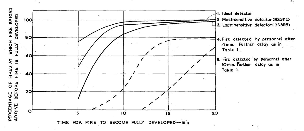
FIG 2. EFFICIENCY OF AUTOMATIC FIRE DETECTORS - NON-RURAL COUNTIES
