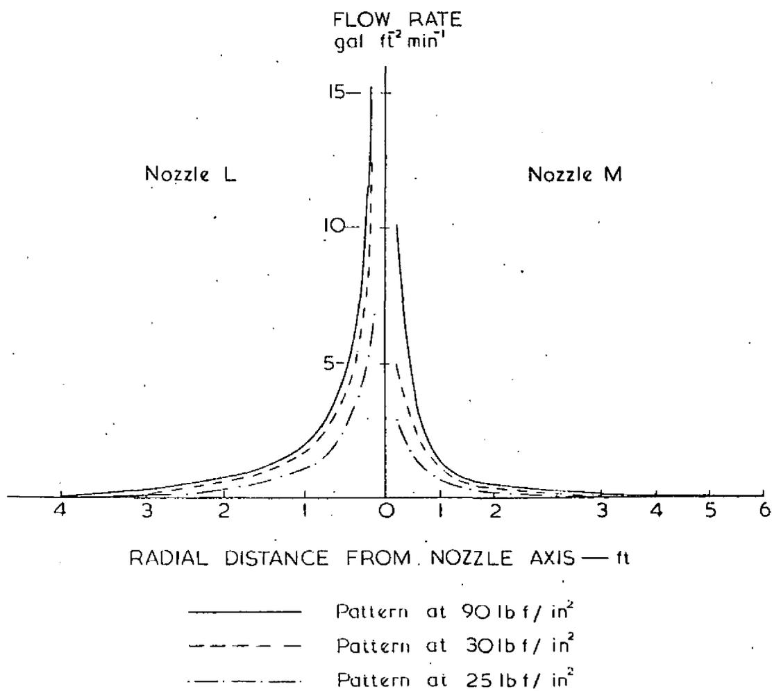
FIG. 4. SPRAY PATTERN, 7'-6" BELOW NOZZLE
