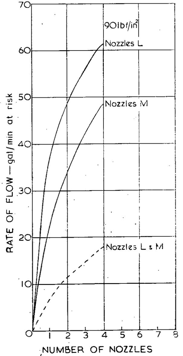
FIG.6. EFFECT OF NUMBER OF NOZZLES
