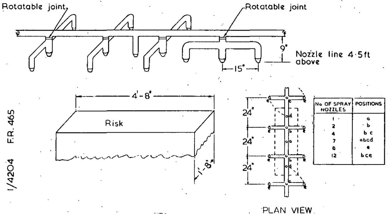
FIG. 2 NOZZLE DISPOSITIONS
