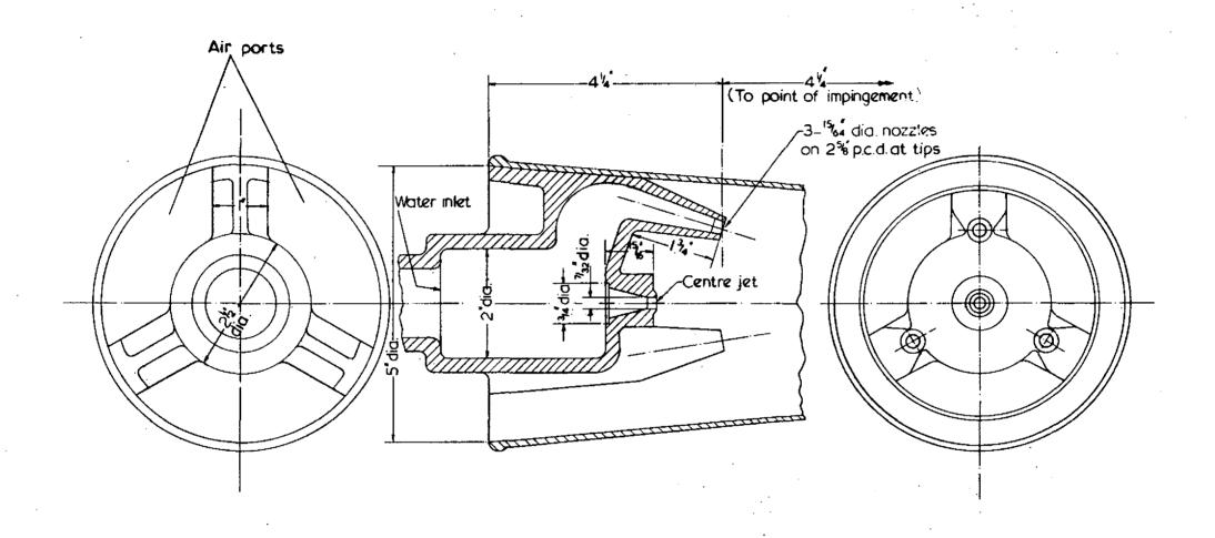
FIG.4. DETAILS OF WATER HEAD OF STANDARD FOAM-MAKING BRANCHPIPE
