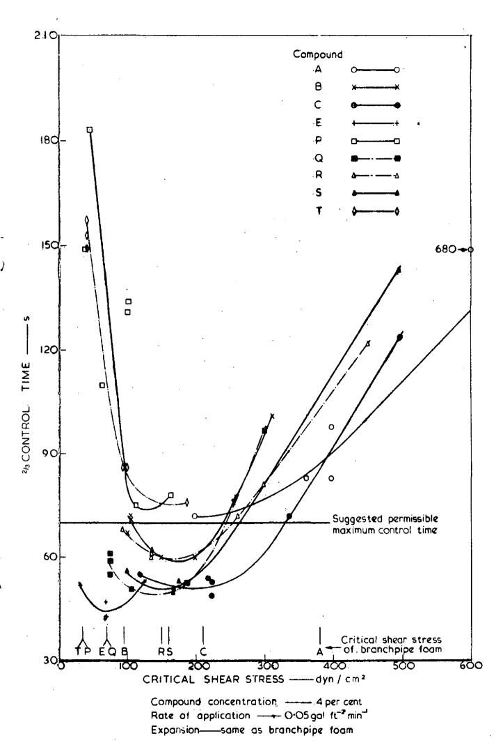
The critical shear stress value of branchpipe foam is indicated at the bottom of the graph
