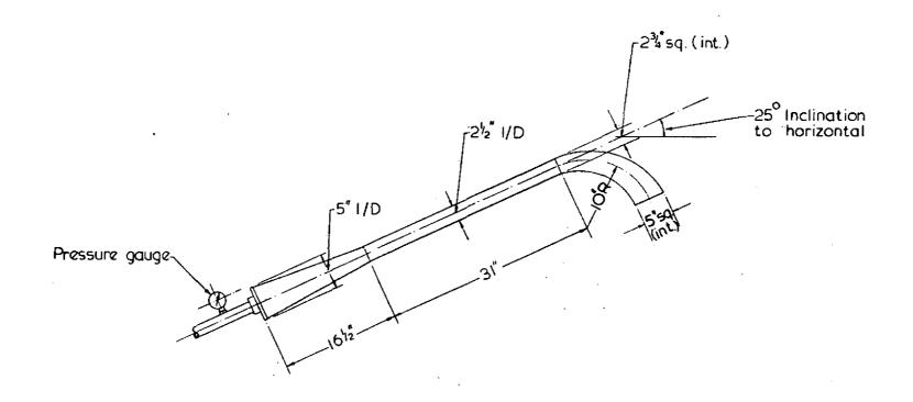
FIG. 3 STANDARD FOAM-MAKING BRANCHPIPE
