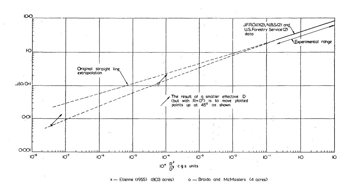
FIG. 1. CORRELATION OF LABORATORY EXPERIMENTAL DATA AND TWO LARGE FIRES
