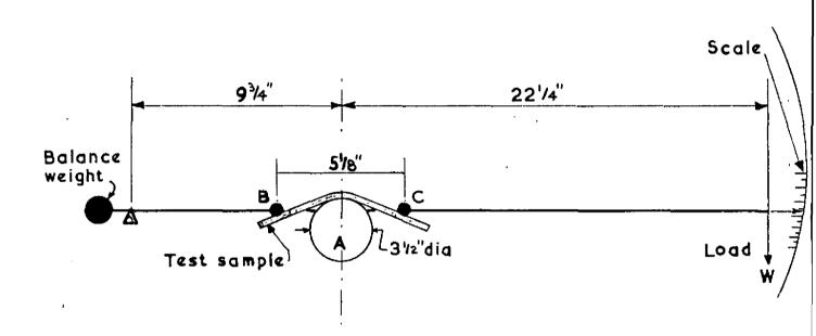
FIG.I. DIAGRAM OF FLEXIBILITY APPARATUS
