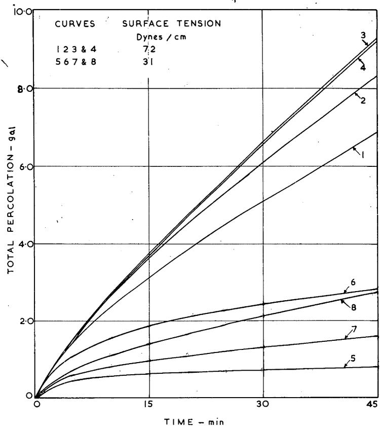
FIG.I. THE VARIATION OF TOTAL PERCOLATION WITH TIME FOR TAP WATER AND WETTING AGENT SOLUTION
