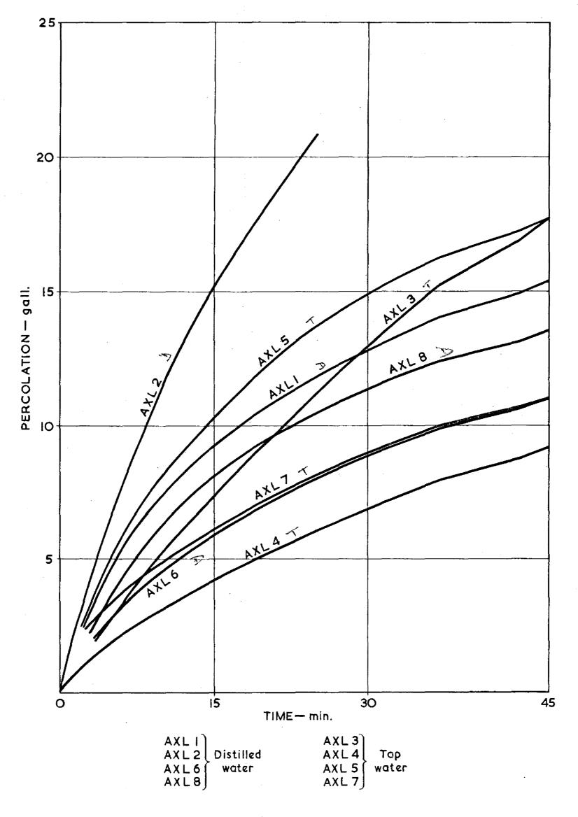
FIG. 1. THE EFFECT OF WATER HARDNESS ON PERCOLATION THROUGH UNLINED CANVASS FIRE HOSE
