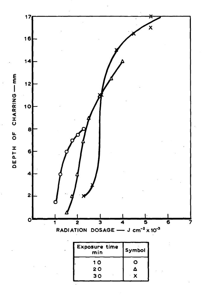
FIG. 1. DEPTH OF CHARRING AND RADIATION DOSAGE
