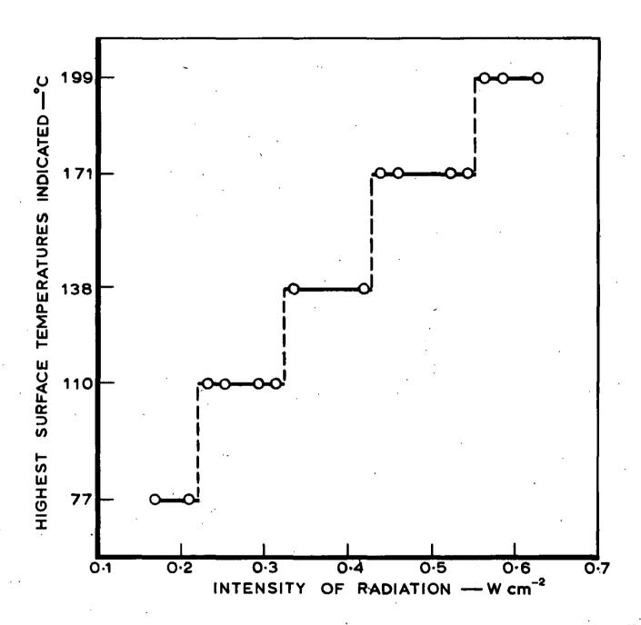
FIG. 6. TEMPERATURE INDICATED BY SENSITIVE PAPERS AFTER 30 MINUTES EXPOSURE
