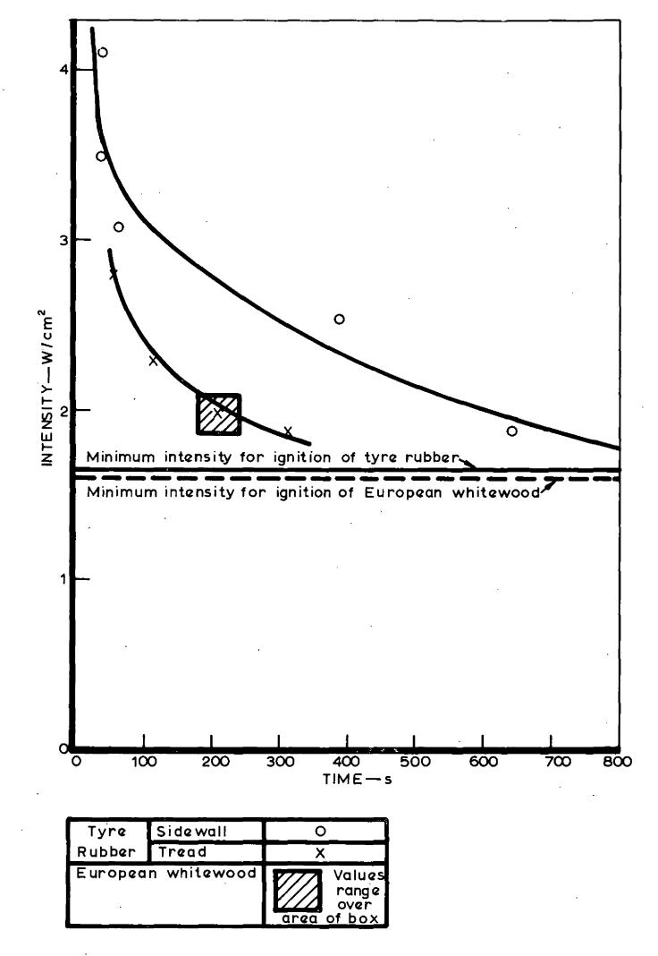
FIG.2. PILOT IGNITION OF RUBBER TYRES
