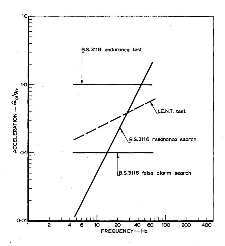
FIG. 2. PROPOSED VIBRATION TEST CURVES
