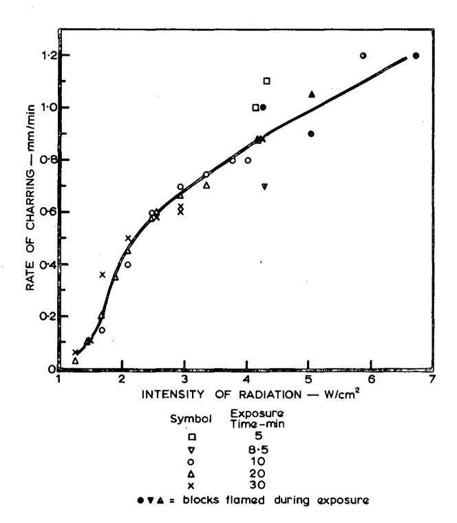
FIG.4. RATE OF CHARRING AND INTENSITY (RECTANGULAR PULSE)
