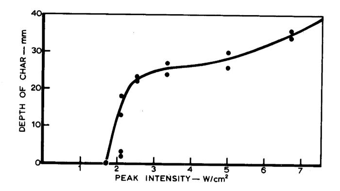
FIG. 2. CHAR PRODUCED BY SKEWED PULSE OF RADIATION
