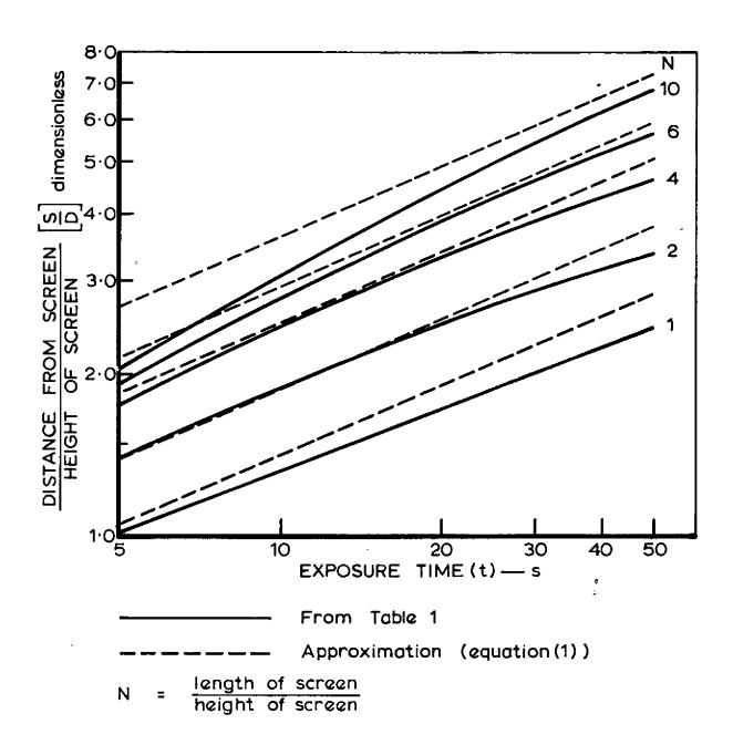
FIG. 1. SAFE DISTANCE FROM WIRED-GLASS SCREEN AND HIGHER INTENSITY FIRE
