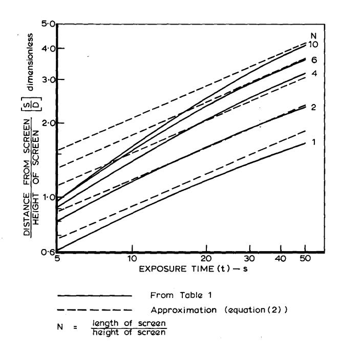
FIG. 2. SAFE DISTANCE FROM WIRED-GLASS SCREEN AND LOWER INTENSITY FIRE
