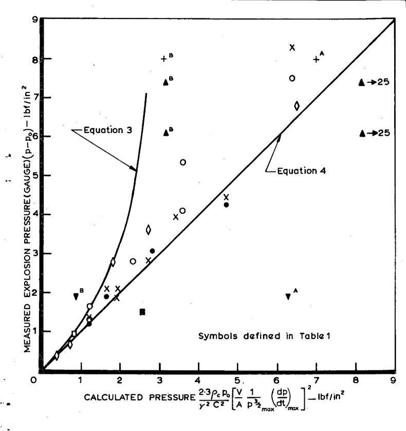
FIG.1 COMPARISON OF MEASURED AND CALCULATED EXPLOSION PRESSURES, BELOW CRITICAL
