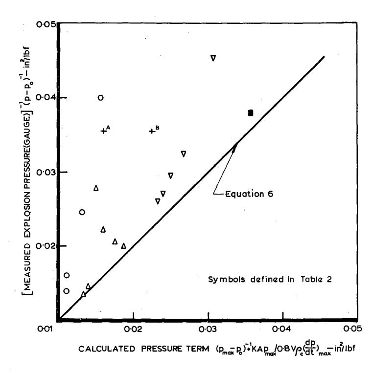
FIG.2 COMPARISON OF MEASURED AND CALCULATED EXPLOSION PRESSURE, ABOVE CRITICAL
