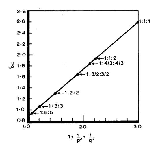
FIG. 1 CRITICAL EXPLOSION PARAMETER FOR RECTANGULAR PARALLELEPIPEDS WITH SIDES 1:p:q
