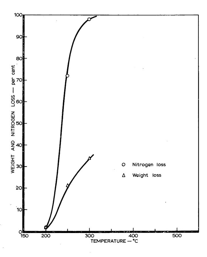
FIG.5. DECOMPOSITION DATA FOR T.D.I. FLEXIBLE POLYETHER FOAM
