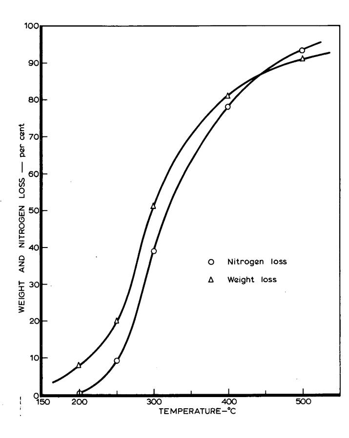
FIG.1. DECOMPOSITION DATA FOR M.D.I. RIGID POLYETHER FOAM
