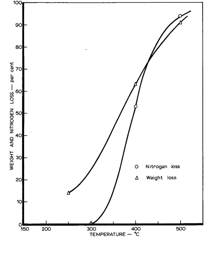
FIG. 2. DECOMPOSITION DATA FOR ISOCYANURATE FOAM
