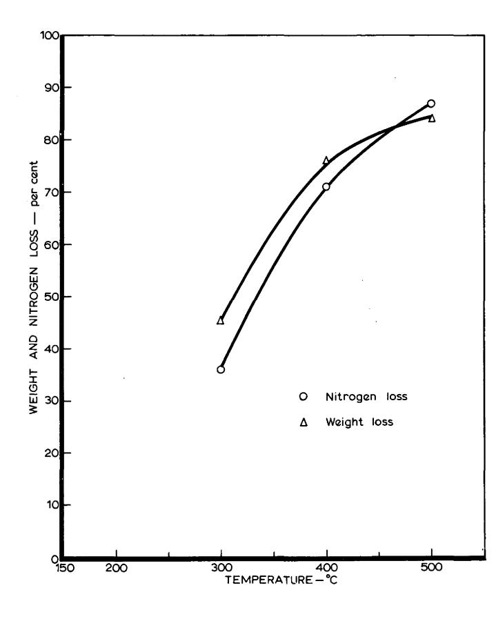
FIG. 3. DECOMPOSITION DATA FOR M.D.I. RIGID POLYESTER FOAM
