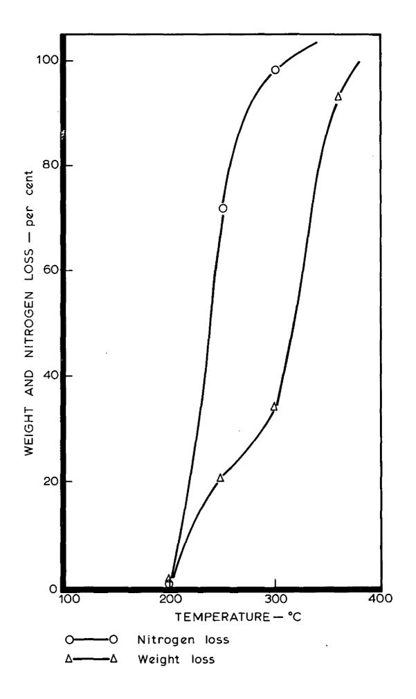
FIG. 4. DECOMPOSITION DATA FOR THE POLYETHER REFERENCE MATERIAL
