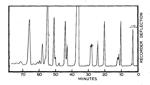
FIG. 8. CHROMATOGRAMS (FID) OF THE DECOMPOSITION PRODUCTS OF THE REFERENCE FOAM AT (a) 600°C AND (b) 900°C
