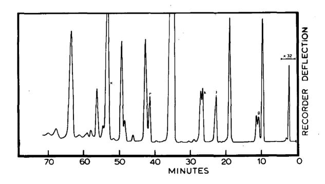
FIG. 5. CHROMATOGRAMS (FID) OF THE DECOMPOSITION PRODUCTS OF FOAM TYPE DAT(a)600°C AND(b) 900°C
