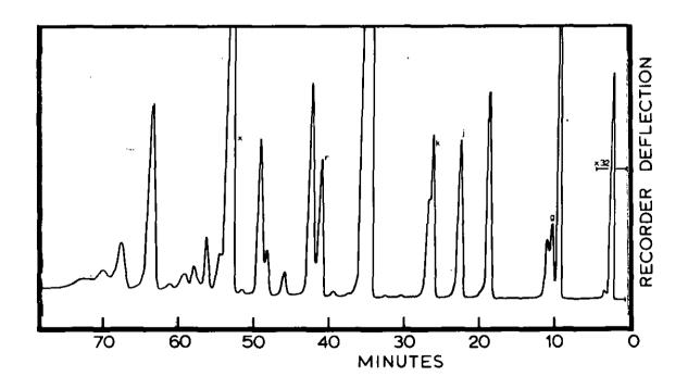
FIG. 6. CHROMATOGRAMS (FID) OF THE DECOMPOSITION PRODUCTS OF FOAM TYPE H AT (α) 600 °C AND (b) 900 °C
