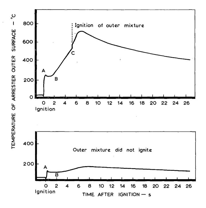
FIG. 8 TEMPERATURE RISES ON ARRESTER SURFACE OBTAINED DURING TESTS ON 1FT3 VESSEL WITH 2 x 4.3" ARRESTERS USING ETHYLENE/ AIR MIXTURE
