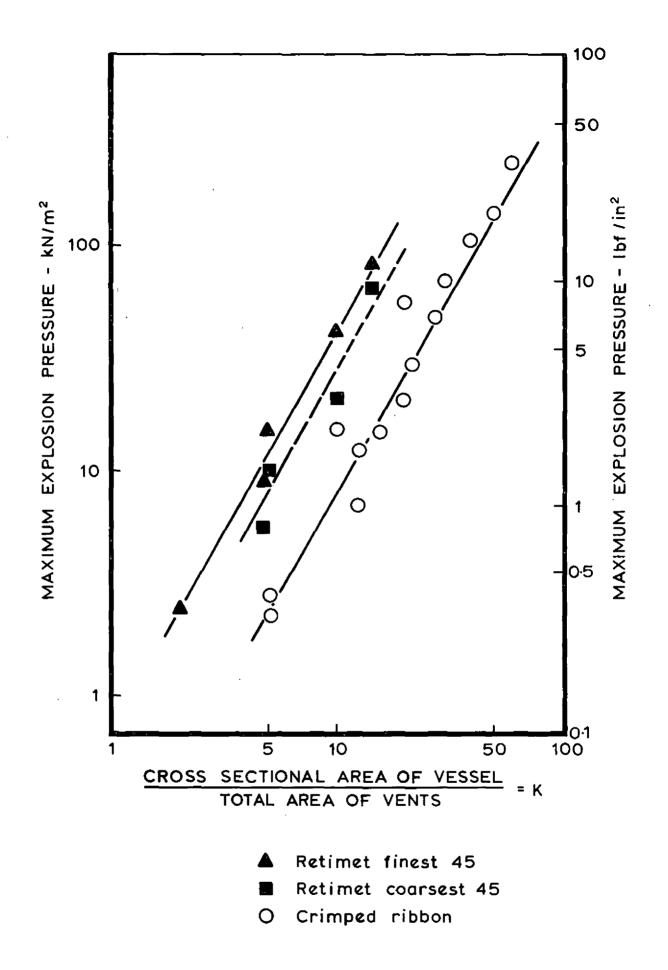
FIG. 7 MAXIMUM EXPLOSION PRESSURE AGAINST VENTING FACTOR FOR RETIMET AND CRIMPED RIBBON USING 4.2 PER CENT PROPANE/AIR
