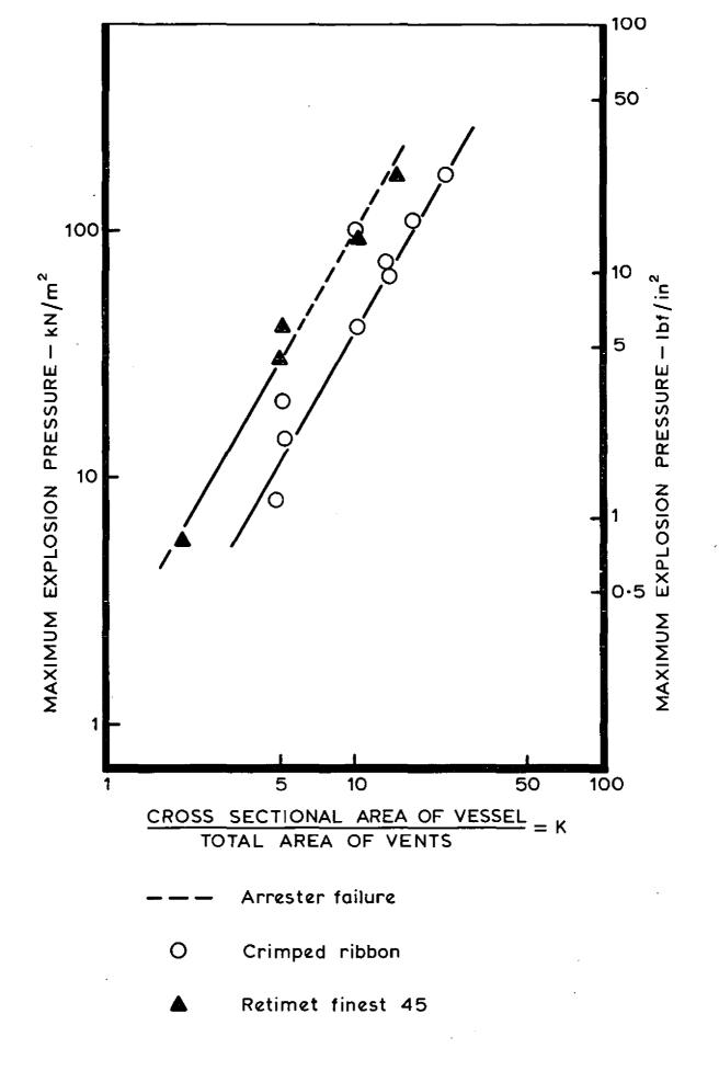
FIG. 6 MAXIMUM EXPLOSION PRESSURE AGAINST VENTING FACTOR FOR RETIMET AND CRIMPED RIBBON USING 6-5 PER CENT ETHYLENE / AIR
