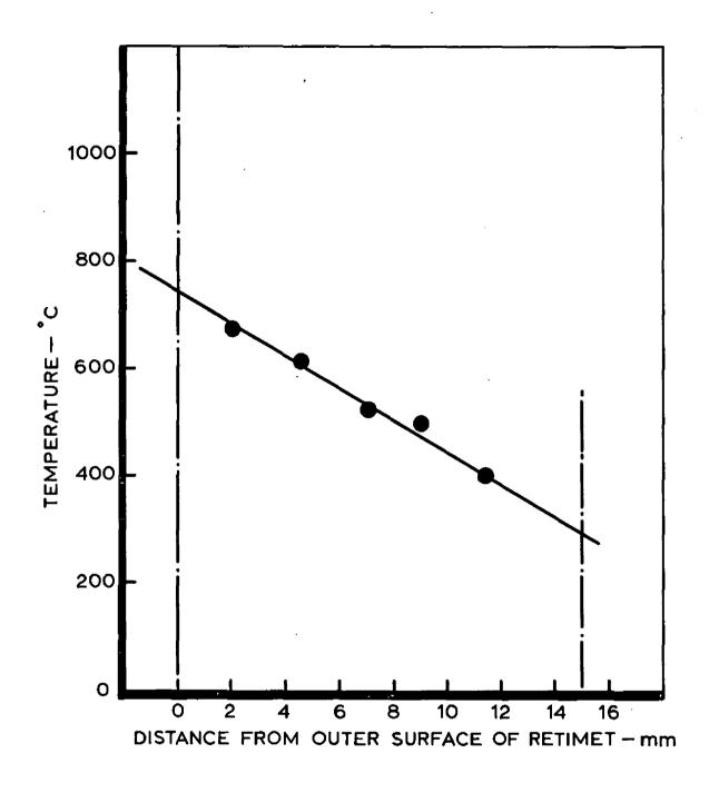
FIG. 11. TEMPERATURE GRADIENT THROUGH RETIMET SPECIMEN WITH FLAME STABILISED ON SURFACE
