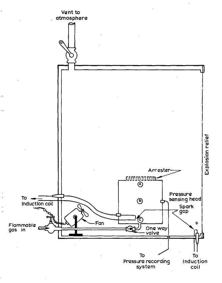
FIG. 3 ARRANGEMENT OF EXPLOSION VESSEL ETC INSIDE TEST CHAMBER
