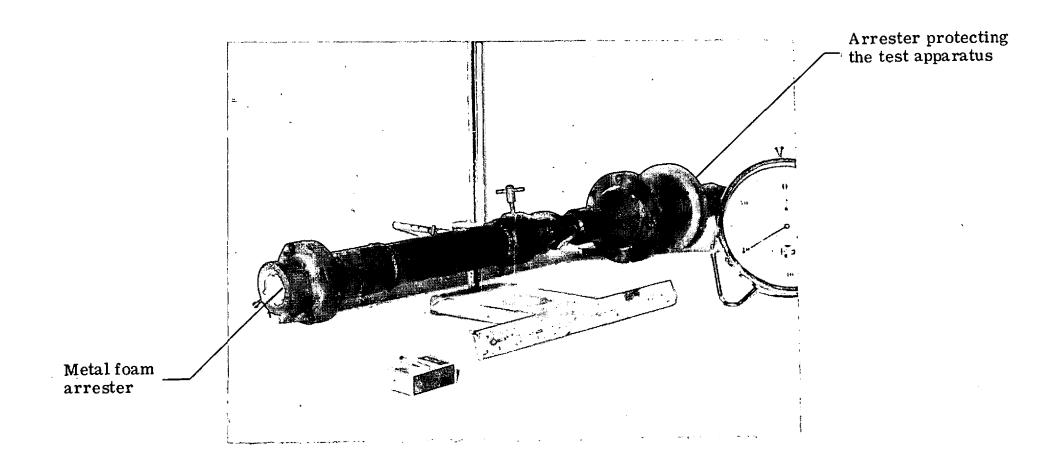
APPARATUS USED IN STABILISED FLAME 'BURNBACK' TESTS
