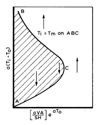
FIG.1. CRITICAL SELF-HEATING CONDITIONS FOR  $\alpha$  [= Hr/K]  $\rightarrow$  O
