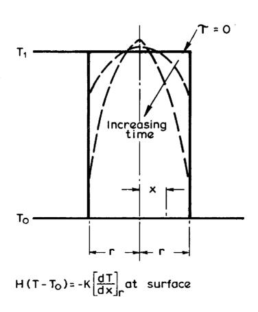
FIG. 2. TEMPERATURE DISTRIBUTION IN RADIALLY SYMMETRICAL "HOT SPOT"
