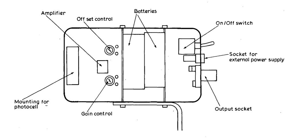
Figure 1 Internal details of radiometer
