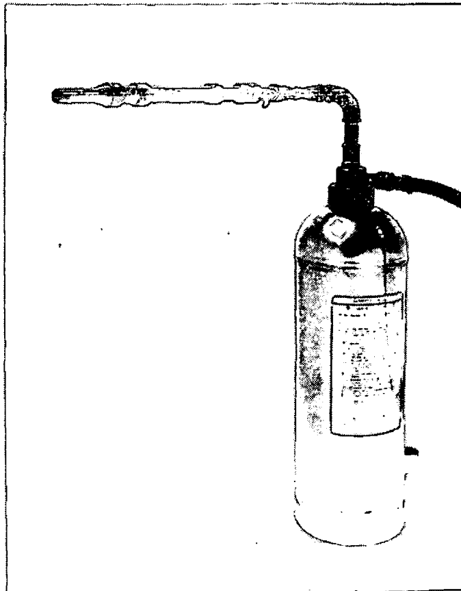
PLATE 3. 5 L/MIN BRANCHPIPE CONNECTED TO EXTINGUISHER, CONTAINING 9.1 LITRES OF 4 PER CENT FOAM SOLUTION AND PRESSURIZED BY AIR LINE CONNECTION
