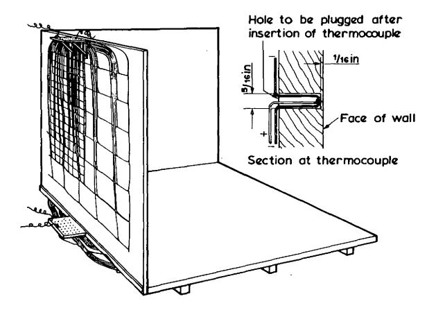
Figure 3 Apparatus for measuring floor and wall temperatures
