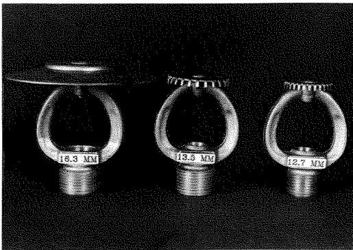
FIGURE 1. Tested upright sprinklers.
